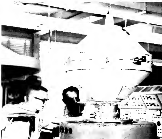
FIGURE A-12.—Explorer VIII being vibration tested. (NASA photograph.)
